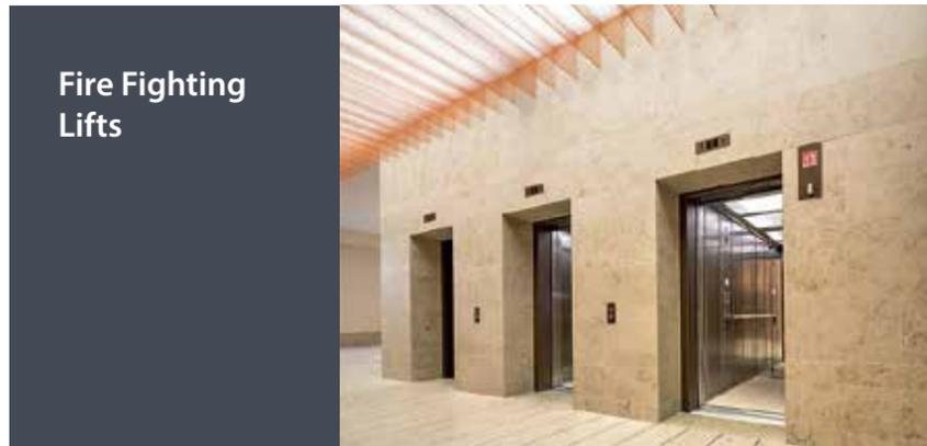
Fire Fighting products are designed according to EN 81.72. in order to be used as both standard lift and as a lift for fire fighters in case of emergency. By turning a key in case of fire - a fire fighter sets the lift in priority and it serves only commanding the lift inside the car.
